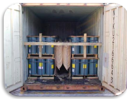
FIGURE 16: Use of inflatable dunnage
