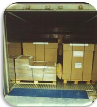
FIGURE 15: Loading of different sized cased goods
