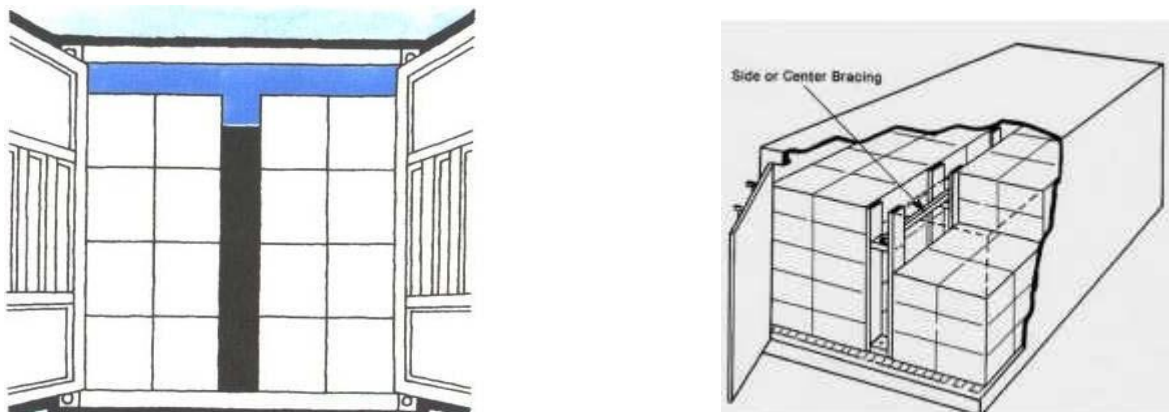
FIGURE 13: Filling void spaces
