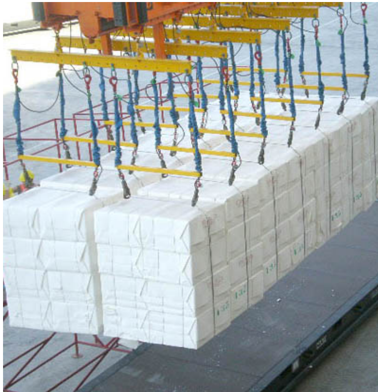
Fig 21: Typical arrangement of lifting gear for unitised woodpulp with pneumatic semi-automatic hooks in operation. (Note two hooks per unit)
