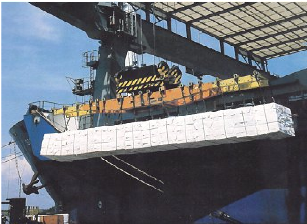
Fig 18: one example of pneumatic release hooks used for top attachment loading and unloading of wood pulp, lumber, plywood and many other products.
