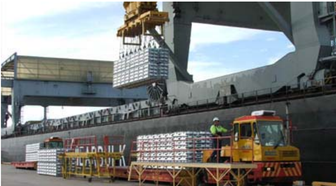
Fig 14: units of aluminium being lifted by flat bands
