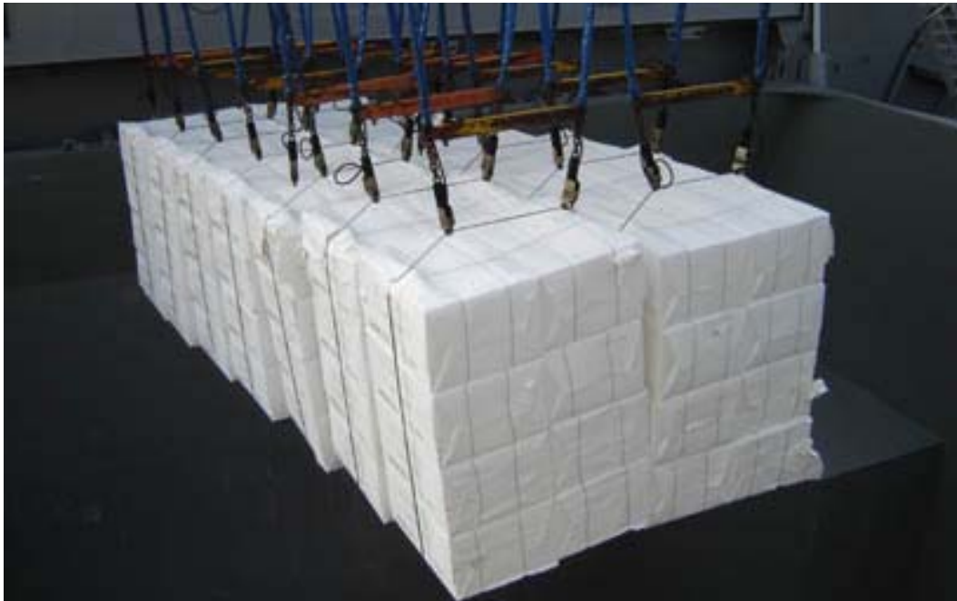
Fig 15: woodpulp unitised for lifting with a round wire lifting system
