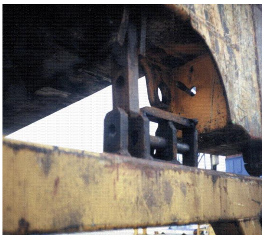
Figure 18 Secondary means of attachment. Pin engaging in link on spreader
