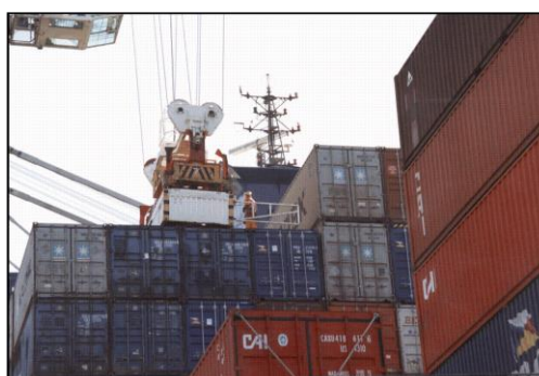
Figure 81 Work with modified half height container with hinged end fences.
