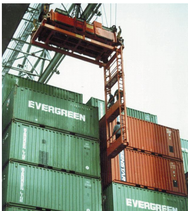
Figure 63 Three tier rigidly attached gondola for working between container stacks.
