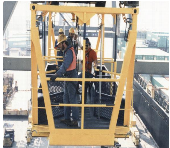
Figure 17 Secondary means of attachment. Chains attached between personnel cage and spreader.
