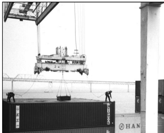
Figure 79 Removing twistlocks while attached to a spreader.
