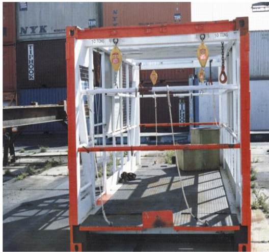
Figure 16 Chains for secondary means of attachment at corners of personnel cage
