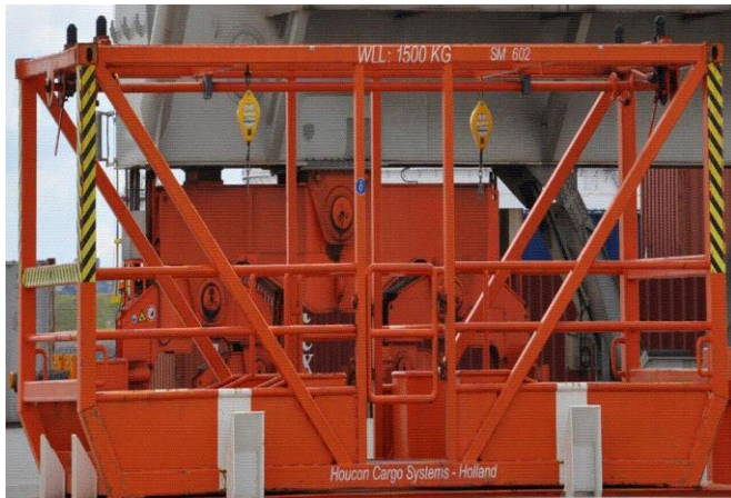
Figure 12 Personnel cage. Note white panels to aid alignment with roll trailer
