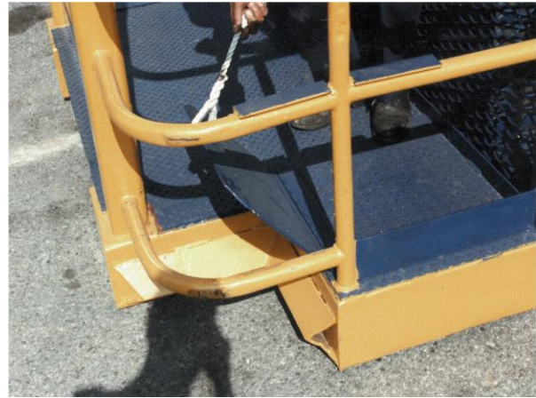
Figure 29 Hinged corner flap closed. Note low hand rail
