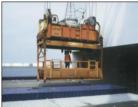
Figure 78 Personnel cage above a stow of containers on a ship.
