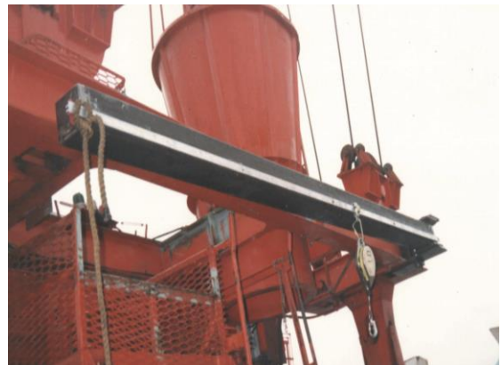
Figure 109 Pivoted beam at each end on a spreader with a fall arrest block attached to a trolley
