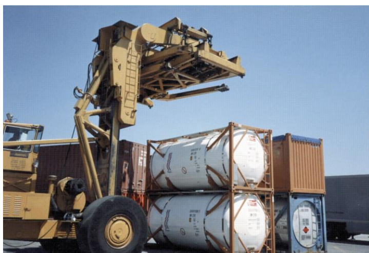
Figure 47 Ladders on ends of tank containers and on reach truck.
