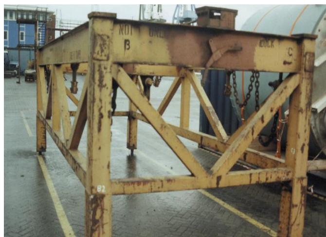
Figure 23 Secondary means of attachment. Pocket on top of an overheight frame into which twistlock in figure 22 locks. Similar pockets can be fitted to personnel cages
