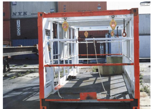
Figure 15 Telescopic personnel cage. Effectively two 10 ft cages mounted at opposite ends of a 20 ft frame. These can be moved apart to work on 40 ft containers.
