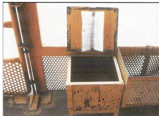
Figure 34 Bins for container securing equipment. The lid can be used as seating when it is closed.
