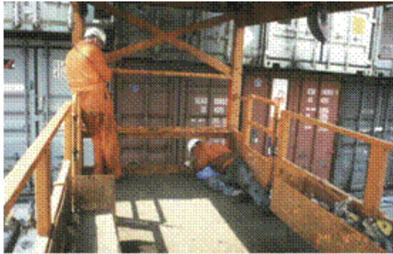
Figure 58 Access to twistlock through end of cage.
