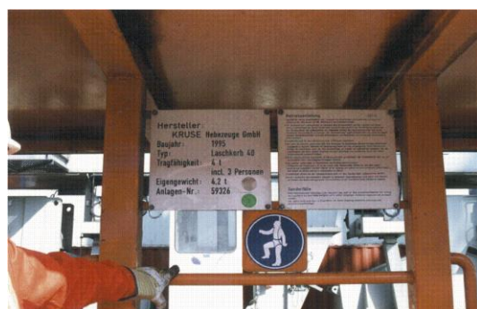
Figure 37 Operating instructions in cage. Note mandatory sign to wear safety harness.
