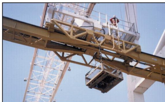
Figure 83 Twistlock basket suspended from spreader.
