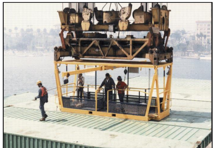
Figure 69 working on tops of containers while secured to landed personnel cage.
