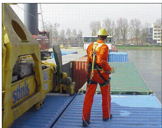
Figure 74 Access to container corner fitting on inland waterway barge protected from landed spreader.
