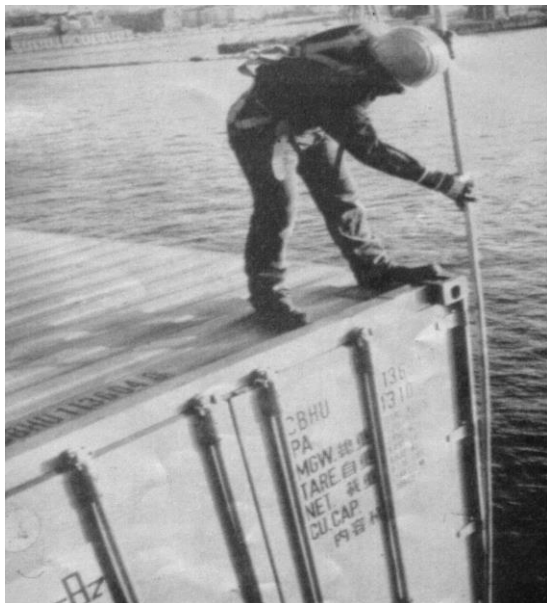
Figure 68 Unlocking twistlocks while secured to landed personnel cage.
