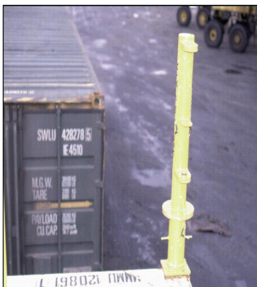
Figure 99 Crane pillar mounted on base unit.
