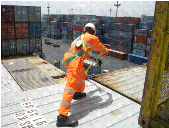
Figure 86 Inserting Top Lock Container Wand while 3 ft from open edge.
