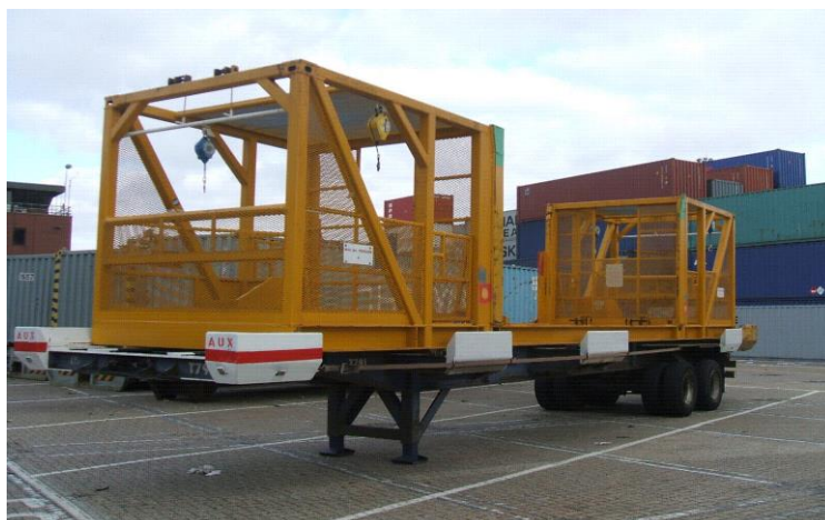
Figure 95 Air draught personnel cage lifted by a 20 ft spreader.
