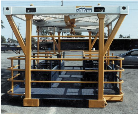
Figure 28 Personnel cage with recessed corners with hinged flaps
