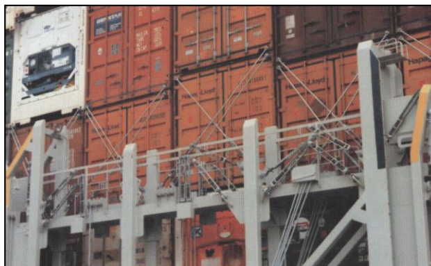
Figure 5 Lashing bridge on ship.
