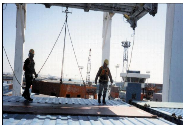
Figure 82 Twistlock basket suspended from spreader.
