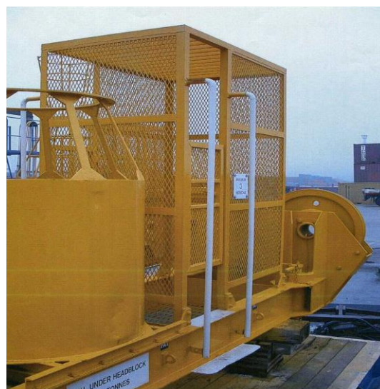
Figure 43 Personnel cage on headblock. Note full protection on sides and top, gate and good access.
