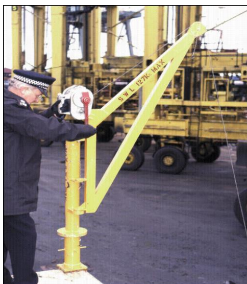
Figure 101 Crane complete with winch.
