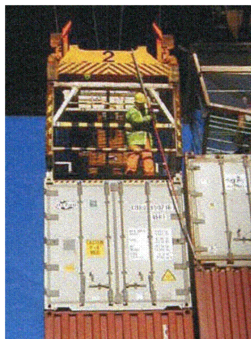
Figure 57 Unlocking personnel cage from above.
