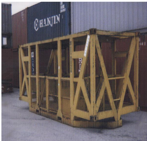
Figure 26 Personnel cage with curved corner recesses
