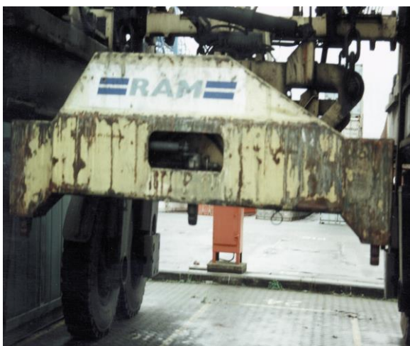
Figure 22 Secondary means of attachment .Additional twistlock at the end of a spreader frame
