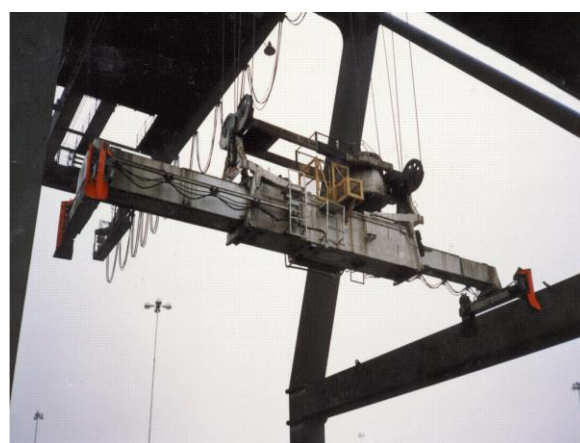
Figure 41 Personnel platform on telescopic spreader
