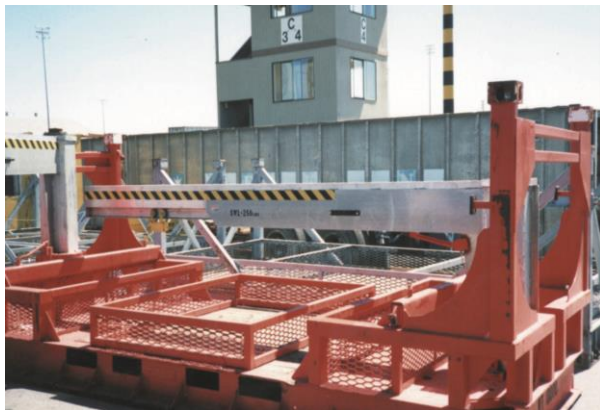
Figure 108 Twistlock basket frame with a pivoted beam at each end on which a fall arrest block can be attached to a trolley
