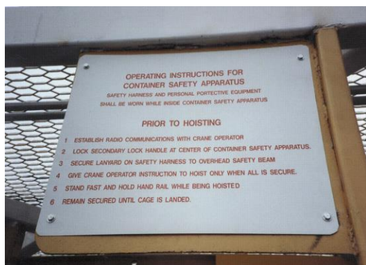
Figure 39 Operating instructions for man riding apparatus (personnel cage).
