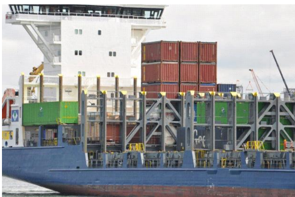
Figure 6 Cell guides and lashing bridge on a ship.
