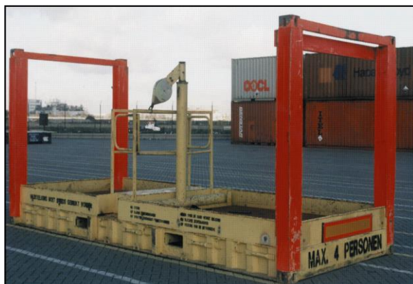
Figure 91 Centre pillar anchorage for personnel protection.
