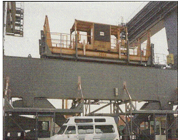
Figure 67 40 ft Double personnel cage stowed on crane cill. The centre section can be lifted separately by a 20 ft spreader.
