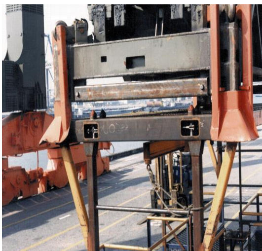
Figure 20 Secondary means of attachment Twistlocks on top of a cage below an additional beam on a spreader.
