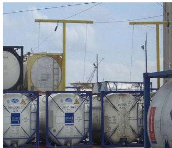
Figure 52 Container top protections in a tank container depot.
