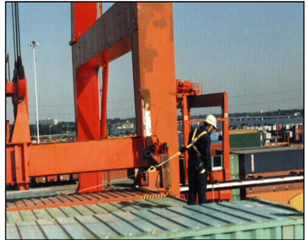
Figure 85 The "Eddie" in use on the tops of containers.
