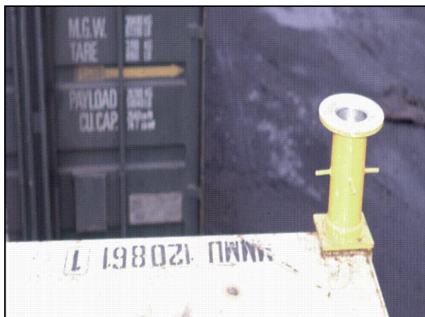
Figure 98 Crane base unit mounted in a container corner fitting.
