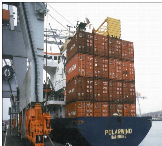
Figure 70 working from landed personnel cage on a feeder ship.
