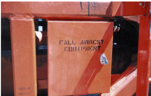
Figure 115 Locker for storage of Fall protection equipment
