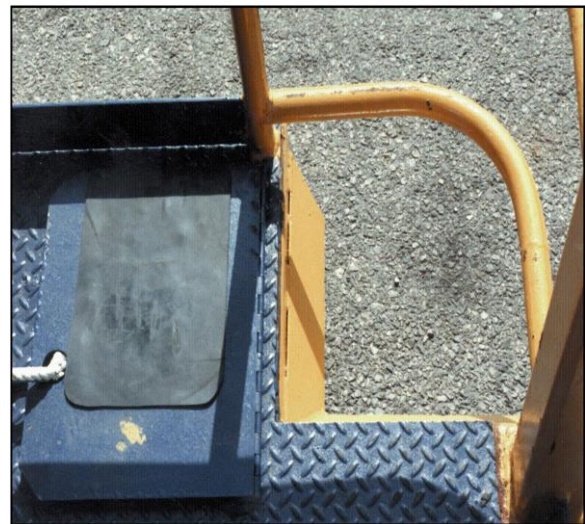
Figure 31 Hinged corner flaps fully open. Note padding on underside of flap.
