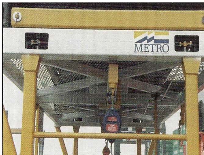
Figure 21 Secondary means of attachment. Twistlocks on top of a cage engaged in an additional beam below a spreader
