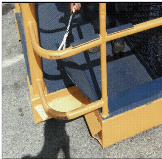
Figure 30 Hinged corner flaps half opened. Note deflectors at edges of recess
