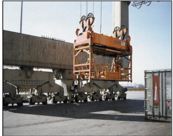
Figure 11 Personnel cage with two gates per side
