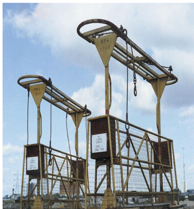
Figure 45 Wire rope supported gondolas. Note platform narrower than top and bottom.
