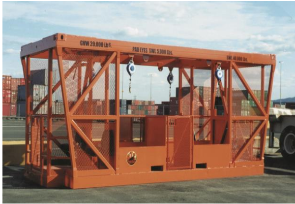
Figure 106 Fall arrest block anchorages to trolleys on runway beams at top of a personnel cage.
