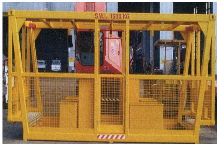
Figure 25 Protected side and ends of personnel cage
