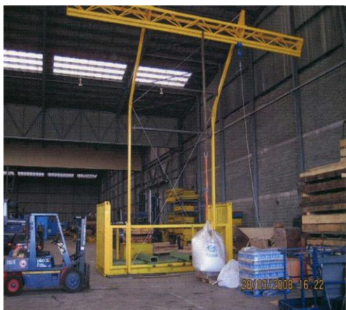
Figure 89 Mobile frames to protect workers on top of containers and similar workplaces.
