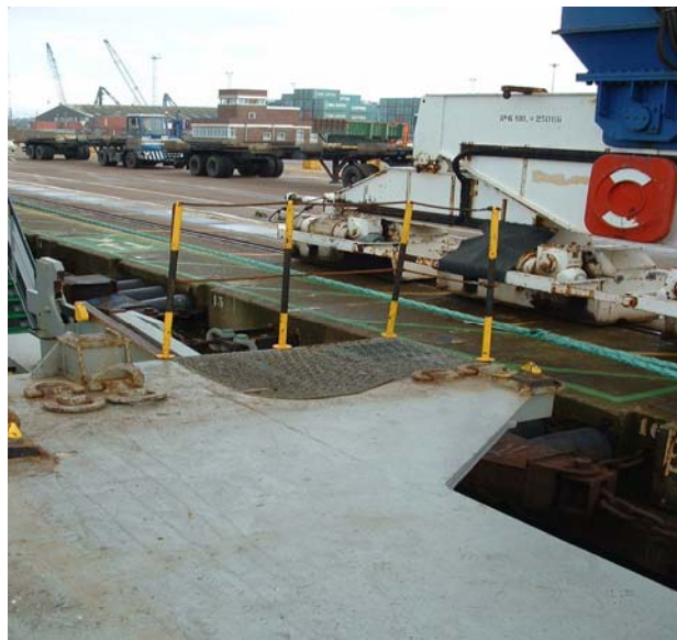
Figure 13: Example of improvements with extra working space and fall prevention
