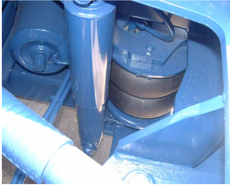
Figure 6 - Rear suspension on a typical container terminal tractor (tug) combining rubber pneumatic suspension (airbag) and hydraulic damper
