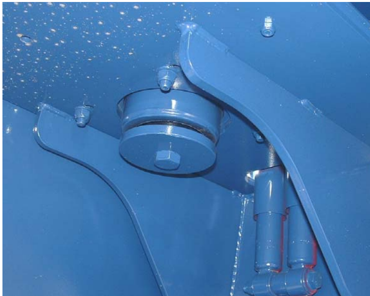
Figure 7 - Rubber block cab suspension with twin dampers
