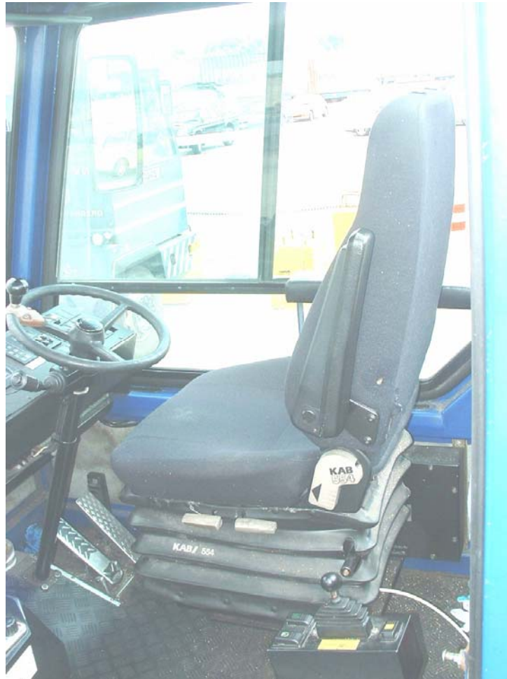
Figure 8 A typical air suspension seat fitted in a terminal tractor
