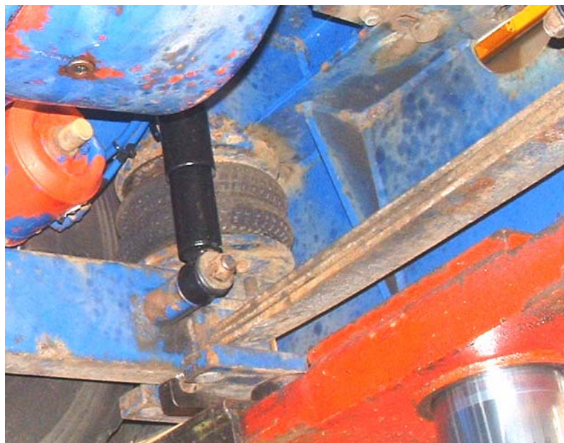
Figure 5 - Front suspension on a typical container terminal tractor (tug) combining rubber buffer leaf spring and hydraulic damper
