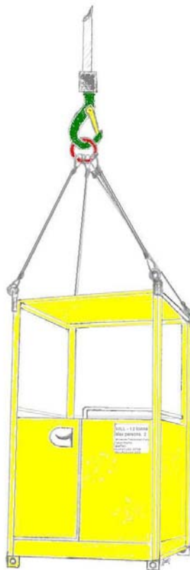
Figure 1 Illustration showing a typical suspended basket
