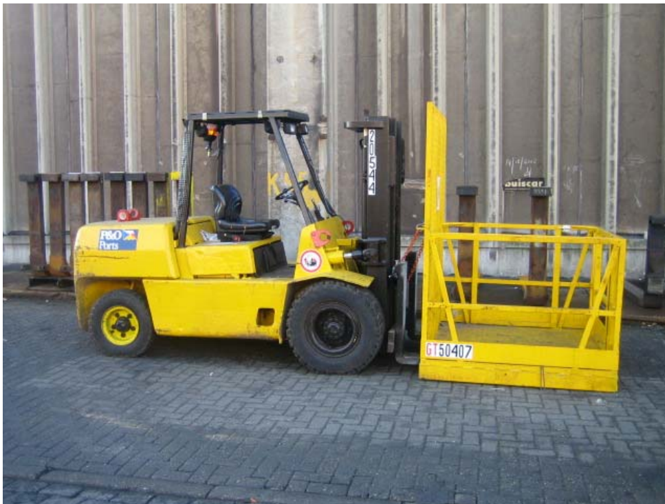
Figure 2 Example of a non-integrated personnel carrier Personnel carrier on forklift truck ( Note - the carrier is also clamped to forks underneath as well as safety chains shown )
