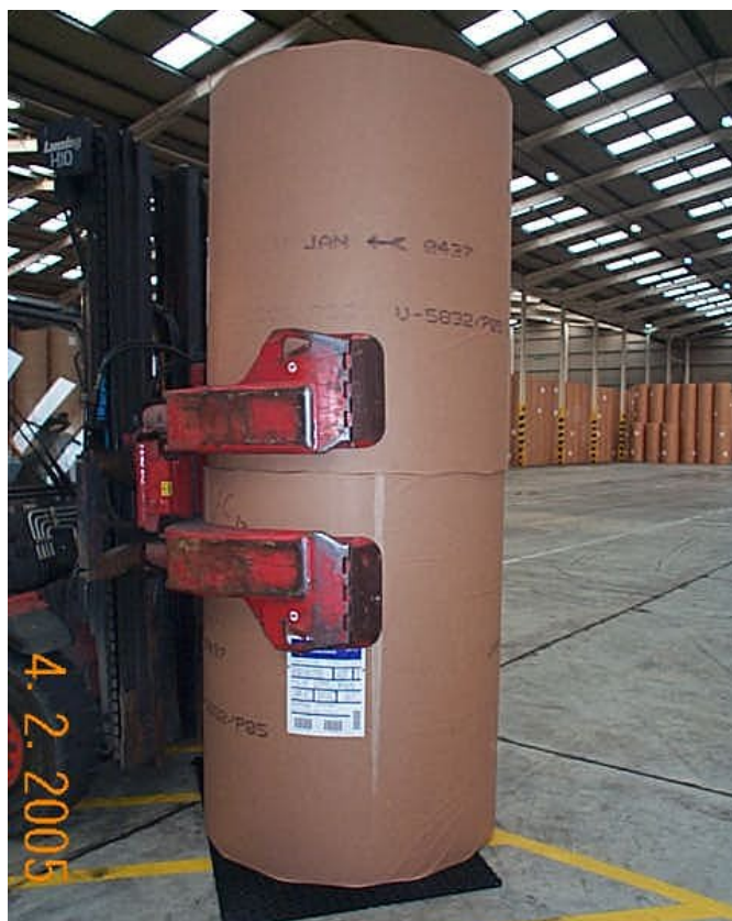
Clamp truck double reel – note protective mat at base.
