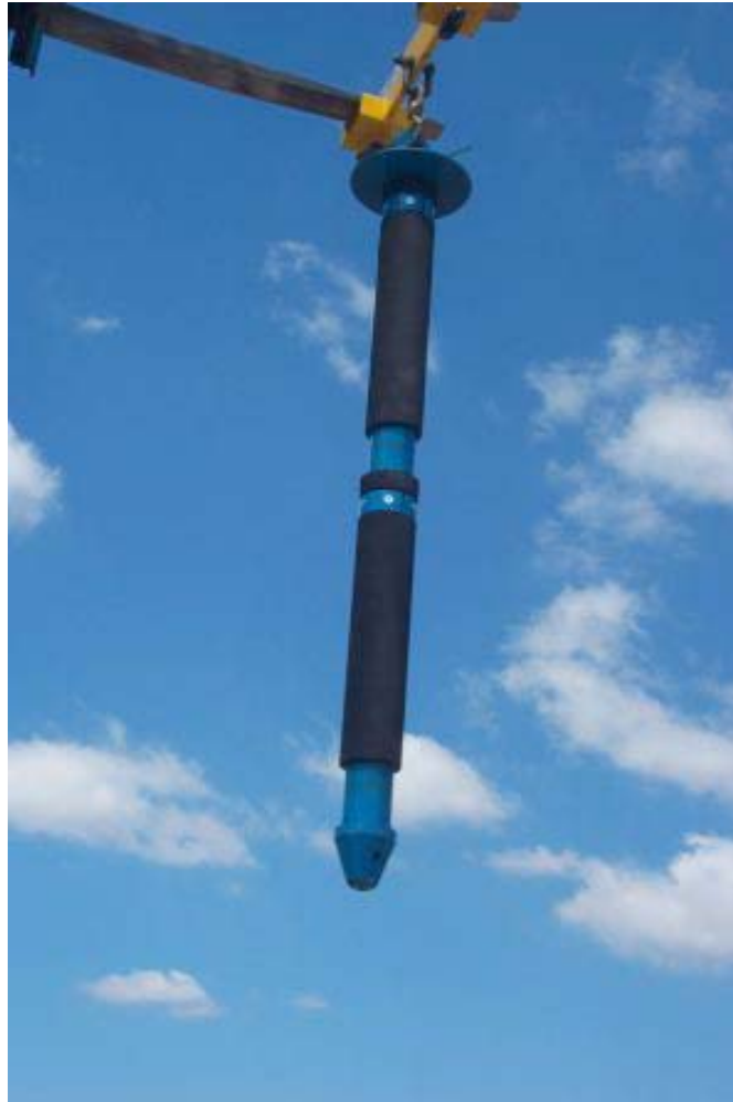
Core probe automatically adjustable for core diameter.
