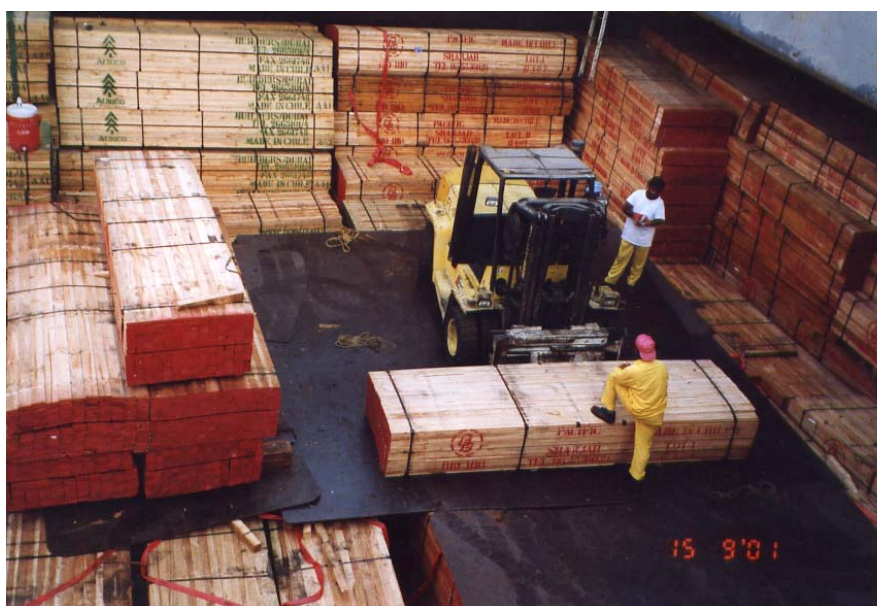
Machine stow: note restriction created by wings.
