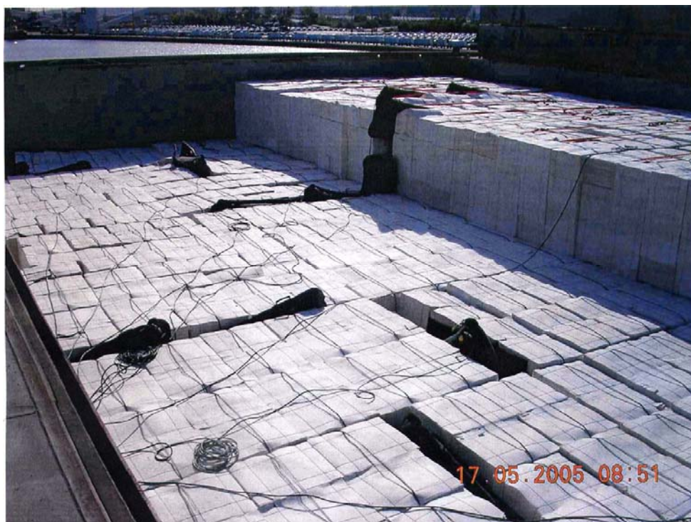
Rubber Airbags in pulp stow connected to a manifold unit
