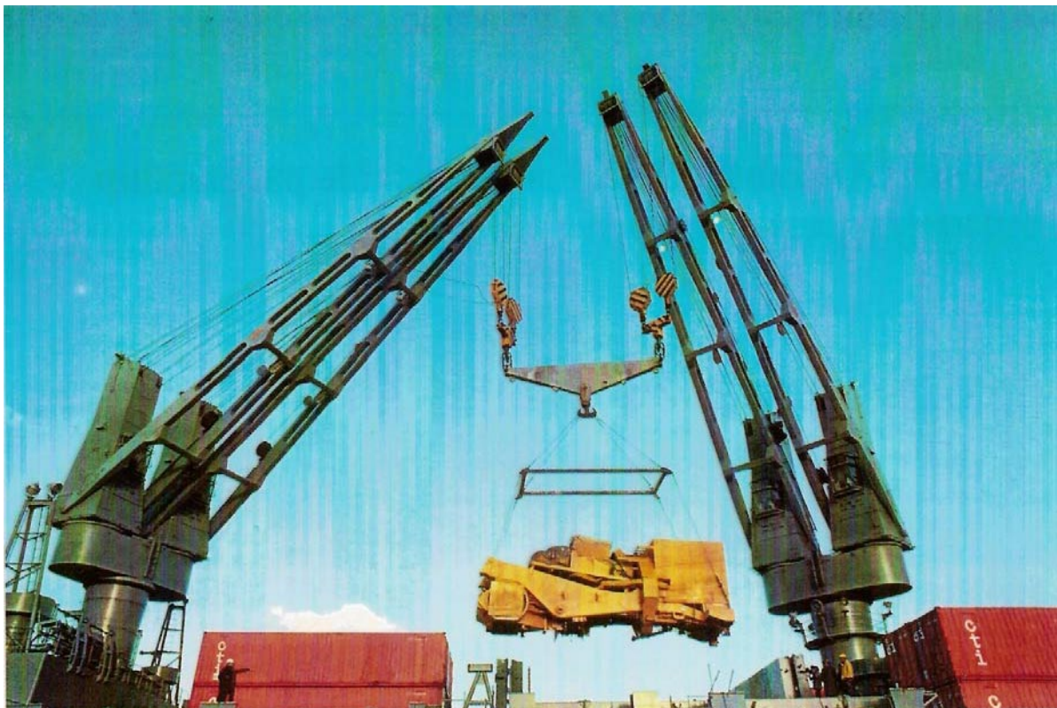
Lifting beams and spreaders in use
