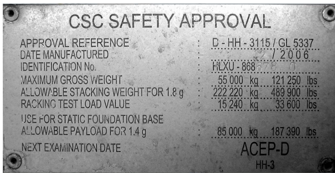
Figure 3 Approved Continuous Examination Program Safety Approval Plate
