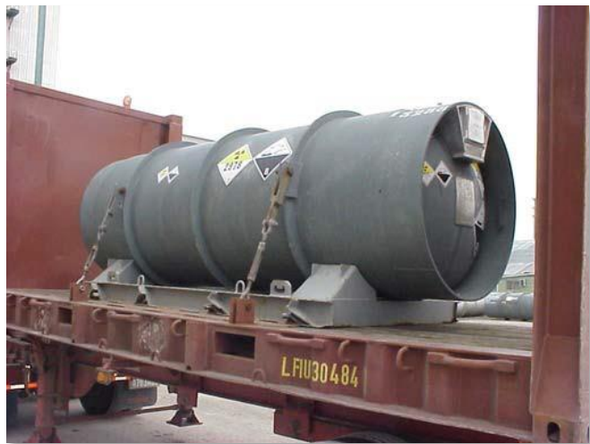
Figure 2 - Uranium hexafluoride [HEX] cylinder ready for transport
