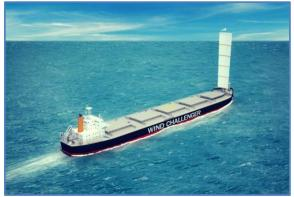
Installation of the hard sail system on merchant ships has the potential to significantly reduce fuel consumption, which in turn will reduce the environmental impact of vessel operation while improving economic efficiency.
