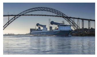
Finnish-based Norsepower has installed the world's first set of tilting rotor sails on board the SEA-CARGO roll-on/roll-off carrier *SC Connector*. The 35-metre Rotor Sails will provide auxiliary wind propulsion leading to reduced fuel consumption, fuel costs and carbon emissions reductions of up to 25%. In favourable wind conditions, the vessel will be able to maintain its regular service speed by sail alone, according to Norsepower.
