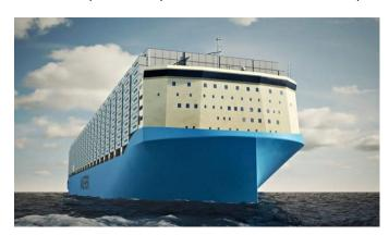
(HHI) with delivery planned for the first quarter of 2024. Most striking is the forward accommodation that Maersk says will enable greater container capacity and improved port efficiency by separating the accommodation and funnel. The funnel is also designed with a reduced footprint and will be located at the stern to maximize cargo capacity.
