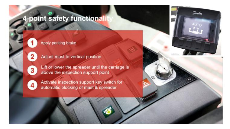
Kalmar's container checker function for its Empty Container Handlers allows the lifting and locking of the container in a safe and ergonomically sound position. This enables effective and safe inspections on all sides and parts of containers, even underneath.
