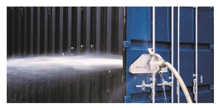
The HydroPen System is connected to the vessel's fire main through standard fire hoses. It is deployed directly to the burning container by the crew who then depart, minimising time in the fire zone. There is no need to attempt to penetrate the container with manual tools and fix spray nozzles inside the burning container.
