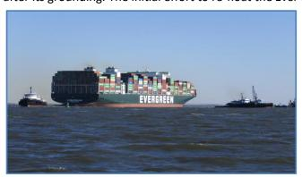
to dislodge the ship recently. Five tugs were used for the operation. The configuration included two tugs pulling on the starboard quarter, one pulling on the stern, and two pushing on the port side.
