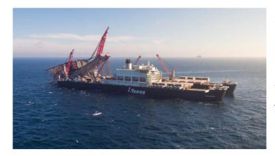
Allseas says the system makes it "fundamentally different" from conventional crane-lifting vessels and the ship's own lifting system. The new system allows for the direct transfer of structures, eliminating the need for support barges. There is also no need to sea fasten the jacket to the beams during transit "due to the vessel's high level of stability, significantly reducing time in the field and lowering the emissions footprint," according to Allseas.
