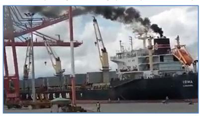
ship's cranes suffered severe damage. It appears that basic measures such as raising the booms of the gantry cranes and lowering the jibs of the ships cranes when berthing on moving along the wharf were not followed.
