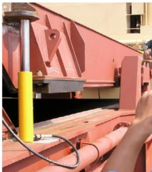
Hatch cover jacking arrangement
