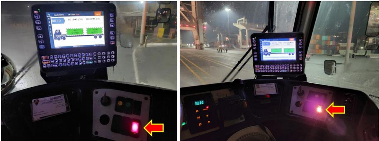
Linking it to the VMT as an added feature has reduced the probability of a container with twist locks being delivered to the yard to ZERO. The system is developed in such a way that it is activated only when the ITV receives vessel discharging container.
