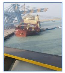
Photos from the scene suggest that before or after the accident, the vessel also listed hard to starboard, towards the wharf. There are several possible explanations for the list changing sides, including improper ballasting, sudden cargo loss, or a vessel switching between sides at the *angle of loll* (the angle of inclination of a vessel under given conditions at which this occurs is known as the angle of loll, and the vessel is said to be in a state of continuous rolling motion).
