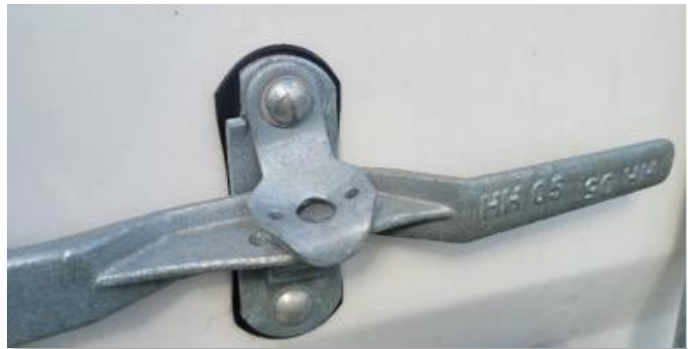
A normal (dumb) container latch
