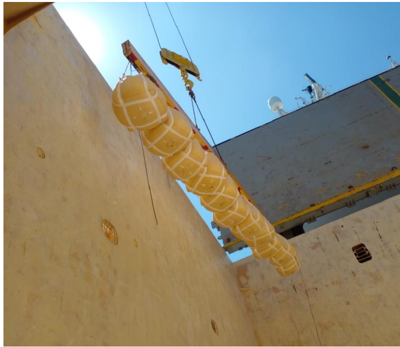
Stevedores were inside the cargo hold, hooking up bags to the spreader beam.
