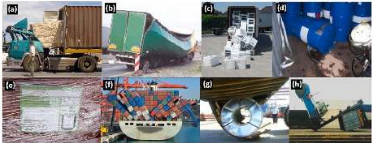
Fig. 1. Consequences of badly packed and secured cargo: lack of longitudinal securing (a); inadequate side wall strength (b); unsecured packages (c); spilled liquid/dangerous goods (d); consequences of insufficient control of humidity, condensation damage (e); consequences of improper deceleration and acceleration, shock failure (f); consequences of the use of unsuitable GTUs, overstressed floor (g); consequences of overloading of GTUs, tipped container handler (h). Source: GTU Code, informative material [1].
