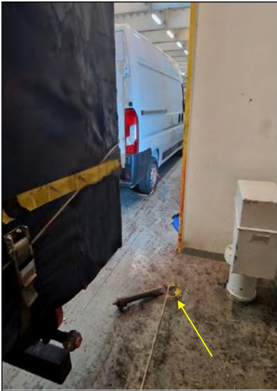
Figure 7: The scene at Deck 3, after the semi-trailer was moved forward to release the AB (one turn buckle seen in position)
