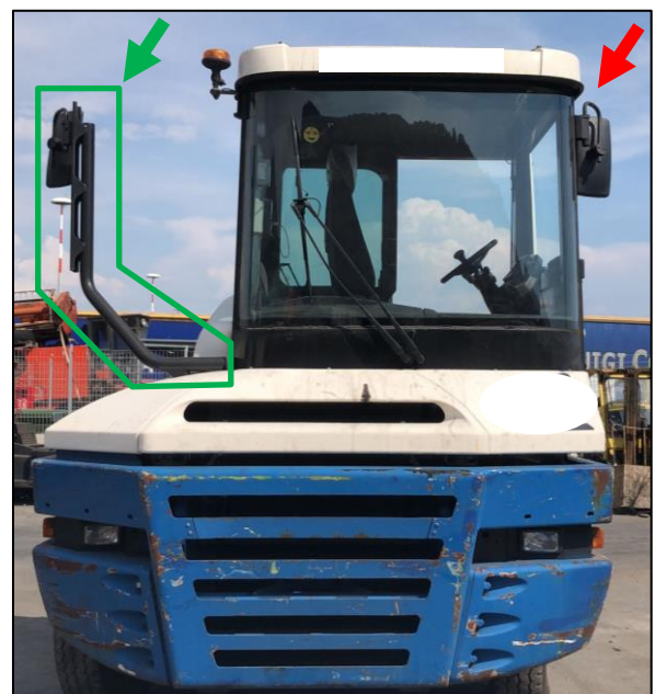
Figure 9: The right-hand side mirror's attachment was designed differently from that on the left-hand side.
