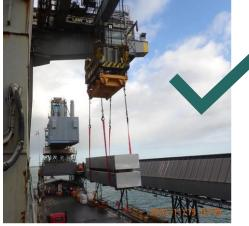
The crane's direction of travel is abeam, not fore-and aft. Abrupt crane movements can always occur, because of a mistake by the crane operator or a technical malfunction. If it happens, the cargo is much more likely to slide out of the slings, if the direction of the cargo is as shown in the in the top right corner.
