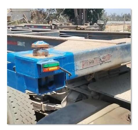
This innovation takes advantage of the air already present in the truck and uses it to perform all the movements necessary for these lashing activities. It secures and tightens the twistlocks avoiding vertical movement of the container during travel.
