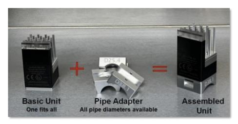
The product consists of a base unit and an adapter that can be exchanged with different sizes matching different pipe dimensions. The device is ATEX Zone 2 certified and can thus be applied in critical environment containing explosive gases. It is also IP65 waterproof and can be cleaned with standard industrial cleaning processes.
