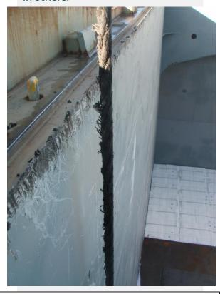
Example of extreme wire damage. Grease marks are clearly visible on the coaming, the wire rope has been dragged over the coaming repetitively.
