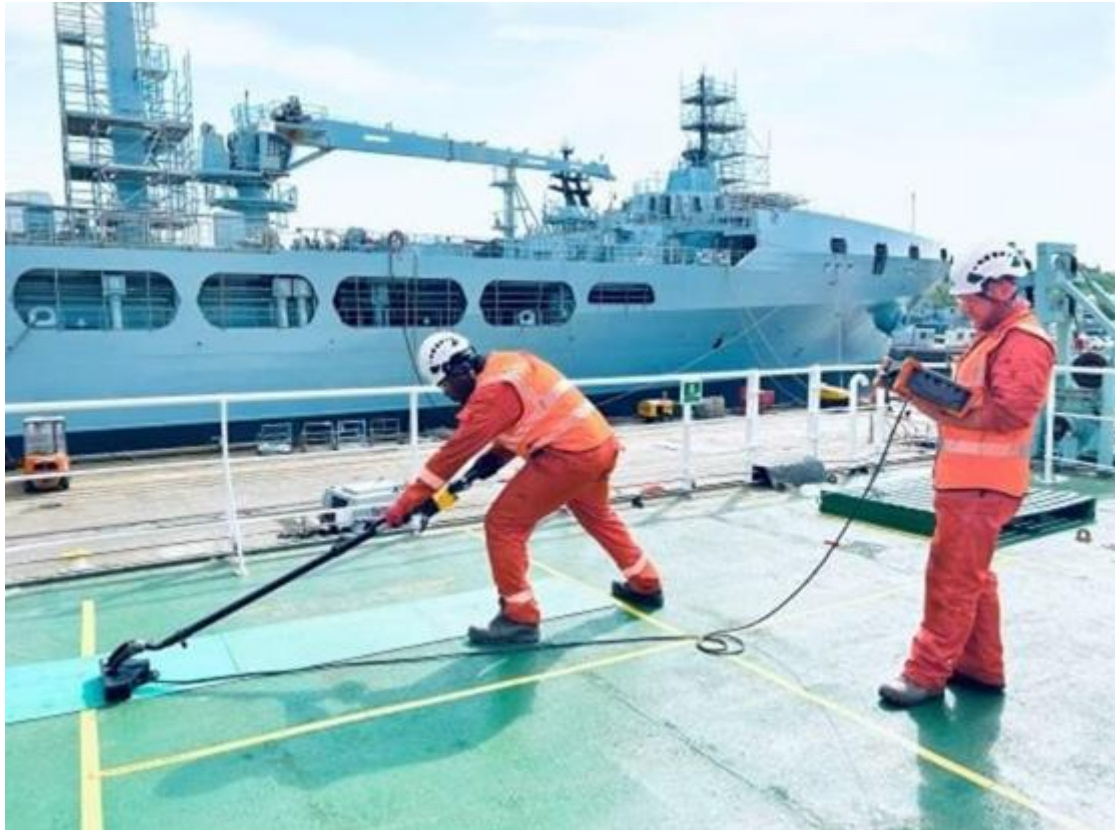
The Lab at Brookes Bell team using CMAP technology to scan a vessel's deck
