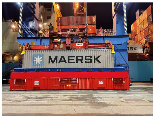
It has magazines that store over 1,000 twistlocks or 2,000 stackers (depending on sizing). This is equivalent to a bay of an Ultra Large Container Vessel.
