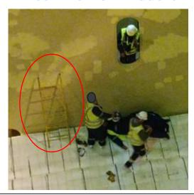
**Incident 1:** A person fell from this ladder, when entering the cargo hold from a manhole. The ladder lacked rubber stoppers at the ends.
