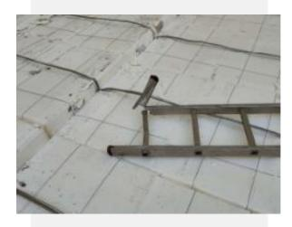
Incident 2: The lowest step of the ladder broke, and a person fell backwards. The ladder was used inside the cargo hold.
