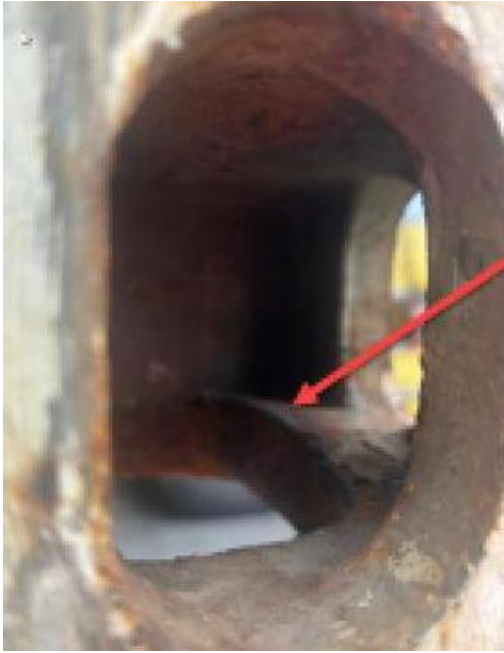
Figure 7 – example defective corner fitting/pocket
