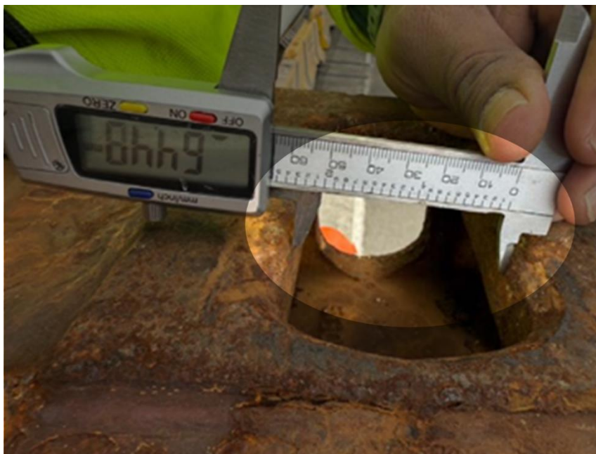
Figure 9 - example inspection of corner fitting aperture
