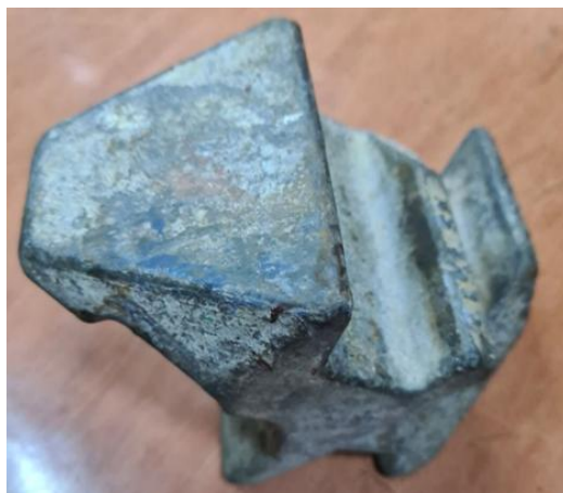
Figure 11 - Twistlock responsible for a work fatality
