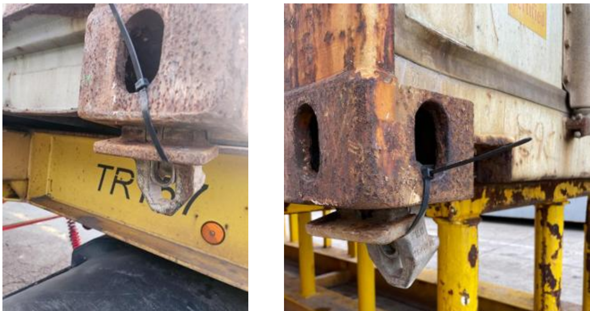
Figure 4 - non-conforming twistlock securing workaround
