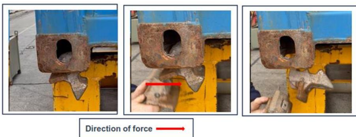
Figure 6 – example of movement giving rise to ‘fall out’ risk from defective corner fitting
