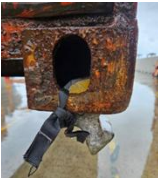
Figure 5 – non-conforming twistlock workaround
