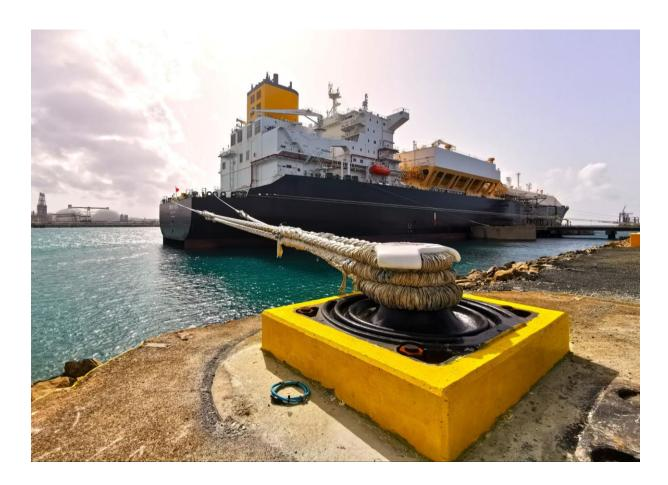
Besides, the Smart Bollard will increase efficiency by gaining a complete overview of the mooring forces in all conditions, which will result in more efficient use of the port. This will, for example, give the possibility to moor larger vessels on quays. Furthermore, it can reduce costs by making data-driven decisions, which can lead to a reduced need for expensive resources such as tugs.
