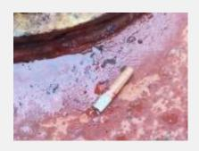
Inside the cargo hold there were big bags with magnesium sulphate heptahydrate fertilizer. This cargo is non-combustible. Cardboard had been wrapped around a steel ladder inside the hold, to protect the bags. It caught fire, and the fabric of some bags were also damaged.
