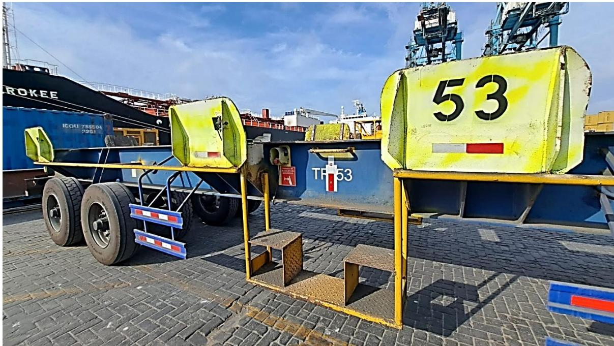
When activated by the tally personnel, these switches block the TT's transmission, fully neutralizing it. This eliminates the possibility of the operator engaging the gear lever while personnel are still within a risk zone.
