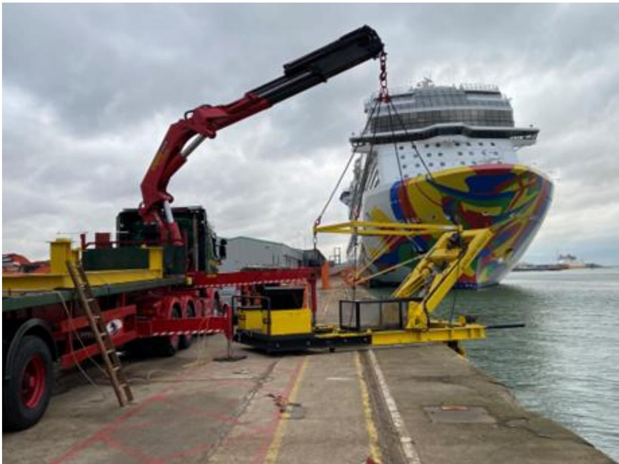
This is a significant and demonstrable advancement on other methods, such as tug pulls, bollard to bollard pulls or modal analysis, none of which are able to fully replicate the working conditions of a mooring bollard or verify working load limit.
