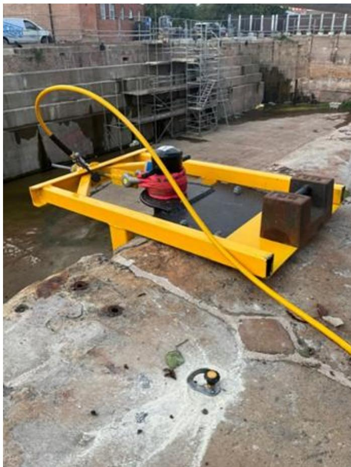
New and innovative methods bring wider exposure, and Bollard Proof has continued to build its client base, with multi-year contracts for testing and increasing levels of testing overseas. To date we have proof load tested in excess of 2,000 bollards across the UK and overseas, in locations as diverse as Guadeloupe & Corsica. The next step is to have our new 250t rig stationed permanently in mainland Europe, with others to follow globally.
