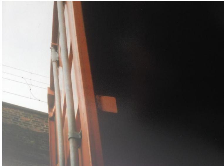
This picture shows the type of external look-a-like fastener that may be used in tampers which break the approved lock bolts. The nut is sealed on to the inside of the door before closure. Door hardware can then be refitted, while in the closed position, with the original, intact Customs seal still attached.
