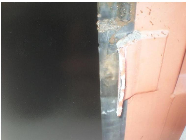
This picture shows an external TIR plate in a state of half tamper. It will be straightened again, after theft or smuggling is completed via the generally unsealed left hand side door
