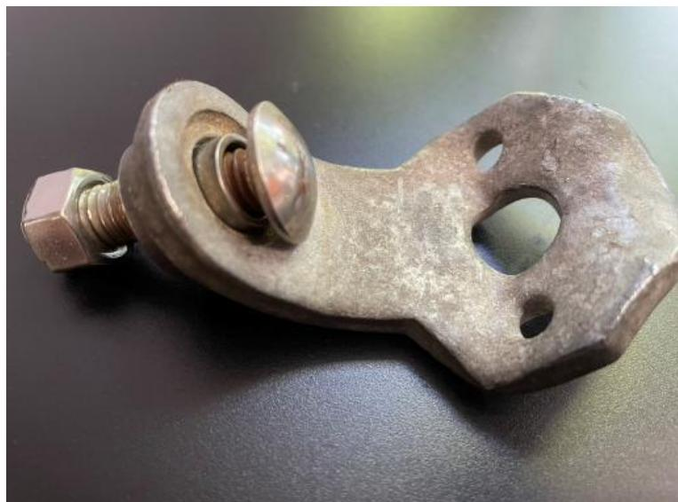
Finally, this picture shows how interior sealing of doors at manufacture could introduce a vulnerability to tampering. This hardware bolt was unscrewed with the nut left on the inside of the door, ready for refitting.
