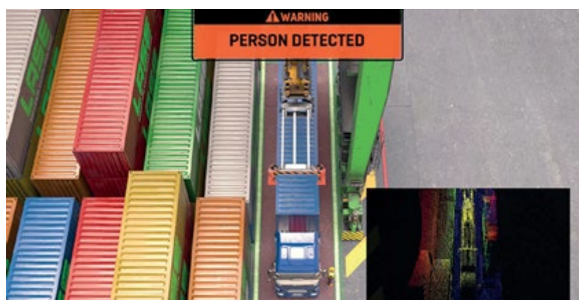
If the target person is outside the safety zone, the yard crane stops
