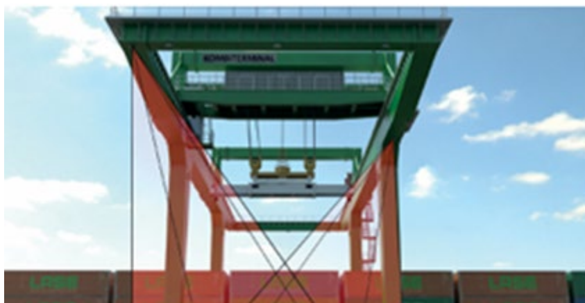
The sensors scan a predefined area above the transfer
