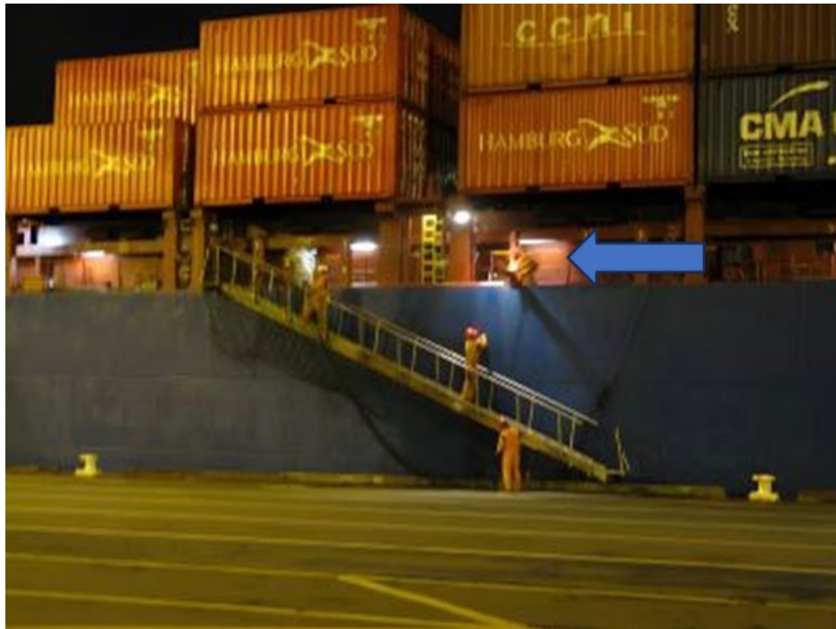
Crew person hanging on the outside of the handrail to help guide the net. There were 6 people involved in this deployment. Only 5 are shown in this picture
