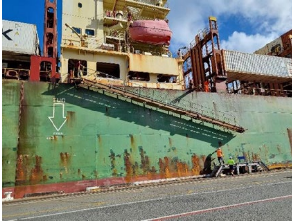
Standing under a suspended load
