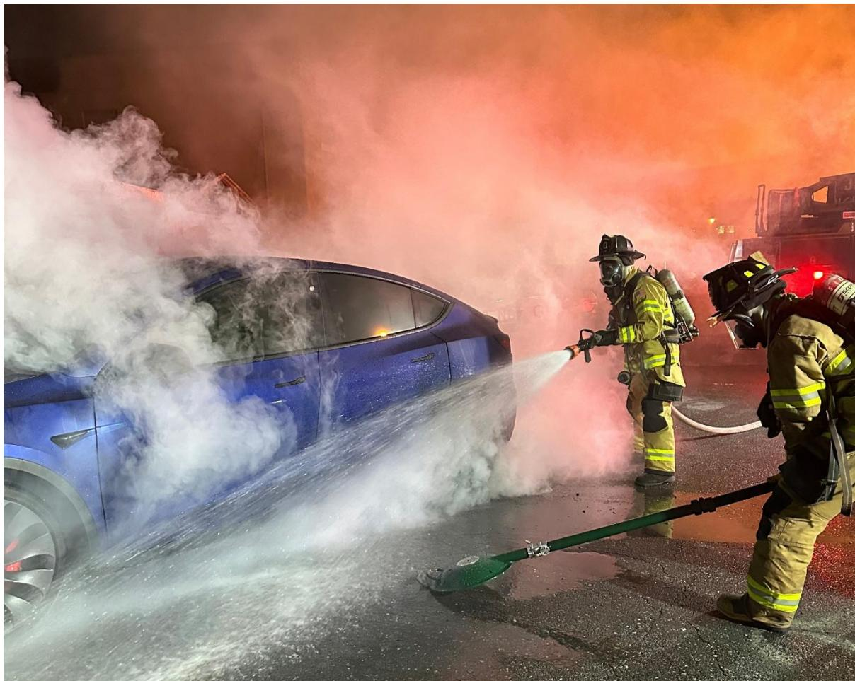
The patented dome shape and 360° flow pattern ensure full coverage of battery casings and surrounding surfaces. Once positioned, the unit delivers a stable, even spray without requiring constant repositioning—reducing exposure for crew members and containing horizontal fire spread. Constructed from powder-coated stainless steel with a slide plate and reinforced handle system, the device is durable, manoeuvrable, and compatible with both marine and land-based firefighting equipment.
