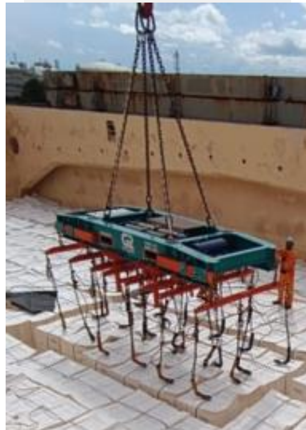
Loading: 6 x 2 pulp units per lift.
